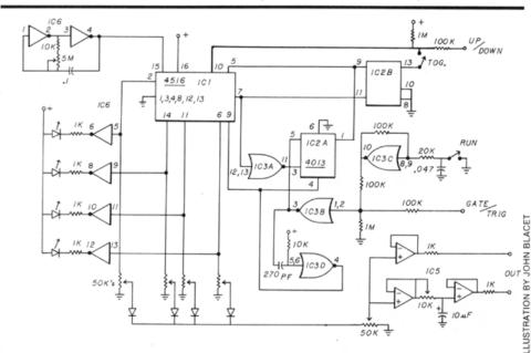
Digital Pattern Generator schematic.
