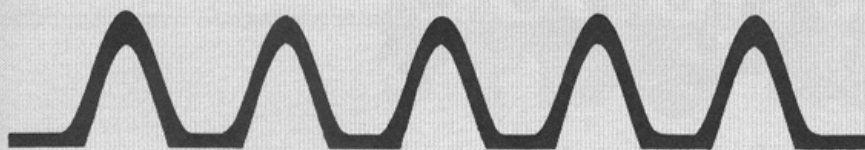
Figure 2. Output of vocal oscillator.
