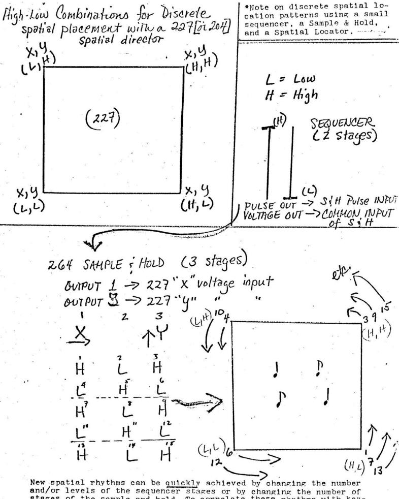
and/or levels of the sequencer stages or by changing the number of stages of the sample and hold. To correlate these rhythms with keyboard passages, for instance, the sequencer could be driven externally with a keyboard pulse.
